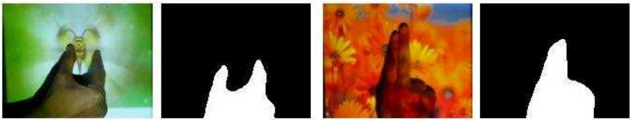
Figure 6.3: Foreground segmentation with hand intrusion using reflectance modelling on plane background
