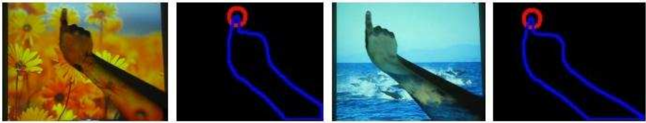
Figure 6.5: Fingertip and type of gesture detection for one finger gestures on plane background
