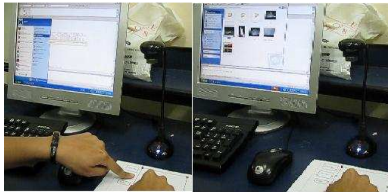
Figure 6.8: Paper touch pad showing operation of left click
