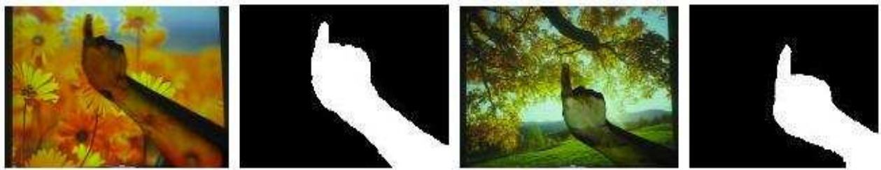
Figure 6.2: Foreground segmentation with hand intrusion using statistical model
