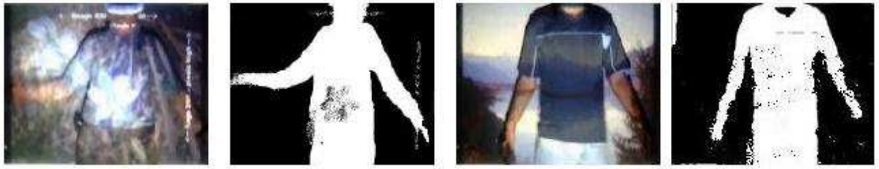
Figure 6.1: Foreground segmentation with full human intrusion using statistical model
