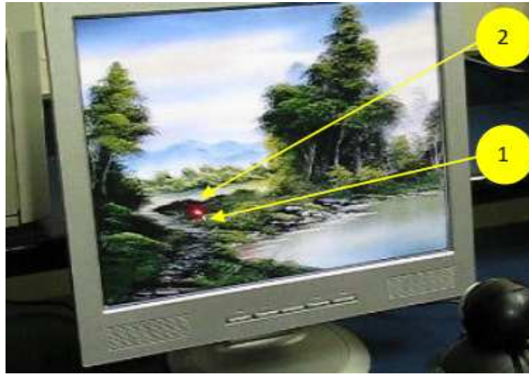
Figure 6.9: Laser pointer mouse showing the recording webcam 1-Mouse cursor and 2-red dot of laser pointer
